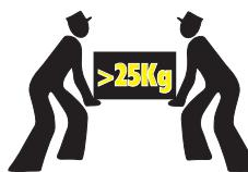
DO NOT handle the machine alone if its weight is over 55lb / 25Kg
