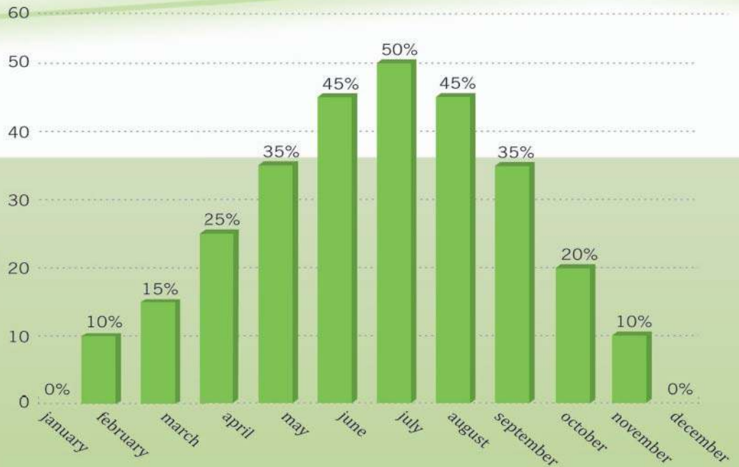
% of savings for the production of domestic Hot Water compared to a condensing boiler
