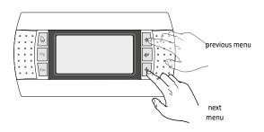
(c) When the desired menu is shown press the key () to enter the menu. Press the key() to return to the menu selection mode.
