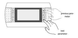
(c) When the desired parameter is shown press the key ( ) to enter the parameter. To exit the parameter and return to the parameter selection mode press the key ( ).
